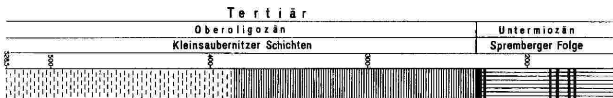
Fig. 6. Schematic section of the Kleinsaubernitz borehole (KIs 1/70). Dashed lines – oil shales; fine lines – diatomites; vertical lines – clays; black – lignites.
