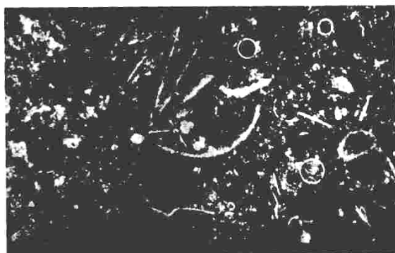
Fig. 6. Parent material: lime-mud supported structure of a bimodal calciturbidite. This carbonate bed-rock microfacies corresponds to transitions from Dvorce-Prokop to Reporyje limestone (Praha Formation). Large bioclasts: planktonic styliolinids - long conical shells with "v"- or "o"- shaped sections; fragmented cephalopod shells - an "u"- shaped section of thin fossil mold with a sparite fill - in a center of figure; thin fragments of a sparite fill - in center of figure thin fragments of trilobite carapaces - undulated sections in lower part of figure.
