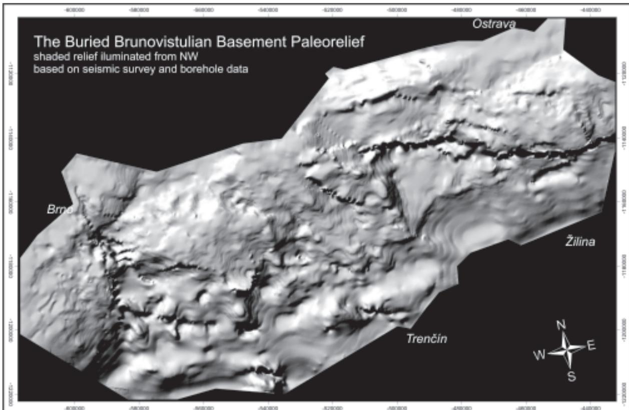
**Fig. 2.** Digital elevation model (shaded relief illuminated from the NW, based on geophysical and boreholes data according to Hubatka, 1997) of buried Brunovistulian (Pre-Paleozoic) basement.
