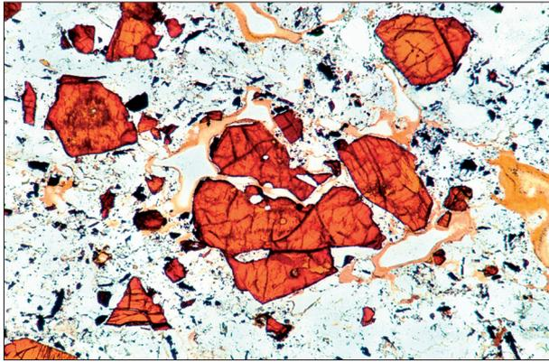
**Photo 7.** Transitional zone from saprolite to the overlying soil (see Fig. 2), western wall of the pit, **depth 55 cm**, PPL. The original saprolite fabric is only marginally disturbed. Coarse pores are clad with micro-laminated kaolinitic clay containing iron oxides,  $700 \times 1050 \mu\text{m}$  in original size.
