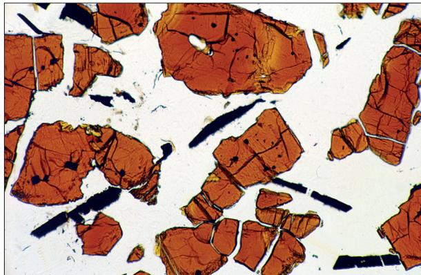
**Photo 3.** Saprolite, western wall of the pit, depth 3.30 m, thin section, plain polarized light (PPL). Reddish-brown iddingsite crystals, partially retaining the crystal shape of the former olivine, can be seen in the upper centre, opaque ilmenites with their characteristic thin tabular cross-sections are found within the bright matrix, 440×660 μm in original size.
