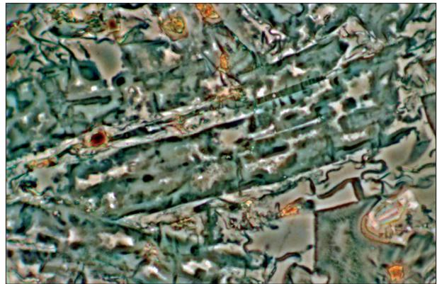
**Photo 5.** Saprolite matrix, western wall of the pit, depth approx. 1 m, phase contrast. The newly formed clay minerals (predominantly kaolinite) can be recognized by their bluish colour against a background of bright pores, which mostly represent dissolution caverns. Plagioclase is totally transformed into kaolinite, the original crystalline shape of the plagioclase, including the polysynthetic twinning is retained (see central part), 240×360 μm in original size.
