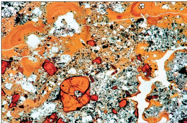
**Photo 8.** Same transitional zone, **depth 30 cm**, PPL. Iddingsite is broken up, mostly mechanically. Ilmenite is predominantly transformed into red iron oxides. The content of yellow-brown clay material increases. Clay cutans are mostly incorporated within the matrix,  $700 \times 1050 \mu\text{m}$  in original size.
