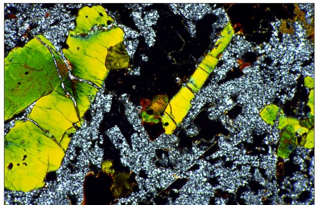
**Photo 12.** Same spot as Photo 11, crossed polars. The matrix of the bauxite bulb consists of gibbsite (fine crystalline, birefringent masses),  $300 \times 450 \mu\text{m}$  in original size.
