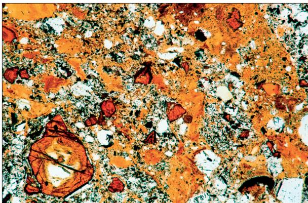
**Photo 9.** Same transitional zone, **depth 15 cm**, PPL. The formation of brown clay and the homogenisation of the material is more advanced here,  $600 \times 900 \mu\text{m}$  in original size.
