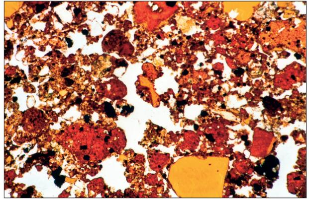
**Photo 10.** Characteristic red-earth-like material with very marked aggregation, northern wall of the pit, depth 5.50 m,  $530 \times 800 \mu\text{m}$  in original size.
