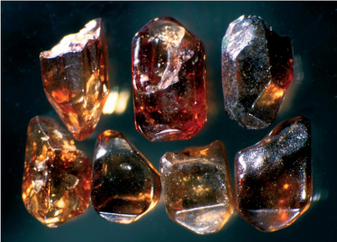
**Fig. 3.** A selection of euhedral zircons (Subpopulation 1) illustrating the clear gem quality and the partly rounded, partly sharp fracture planes. Upper row: D-type and lower row: different S-types after Pupin (1980). Photomicrograph in reflected light (field height ca. 9 mm).
