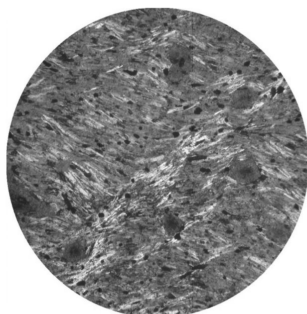
Fig. 7. Microphotograph of sanidine microstructure of trachytic rock. Cross-polarised light enhanced by a  $\lambda$  plate.
