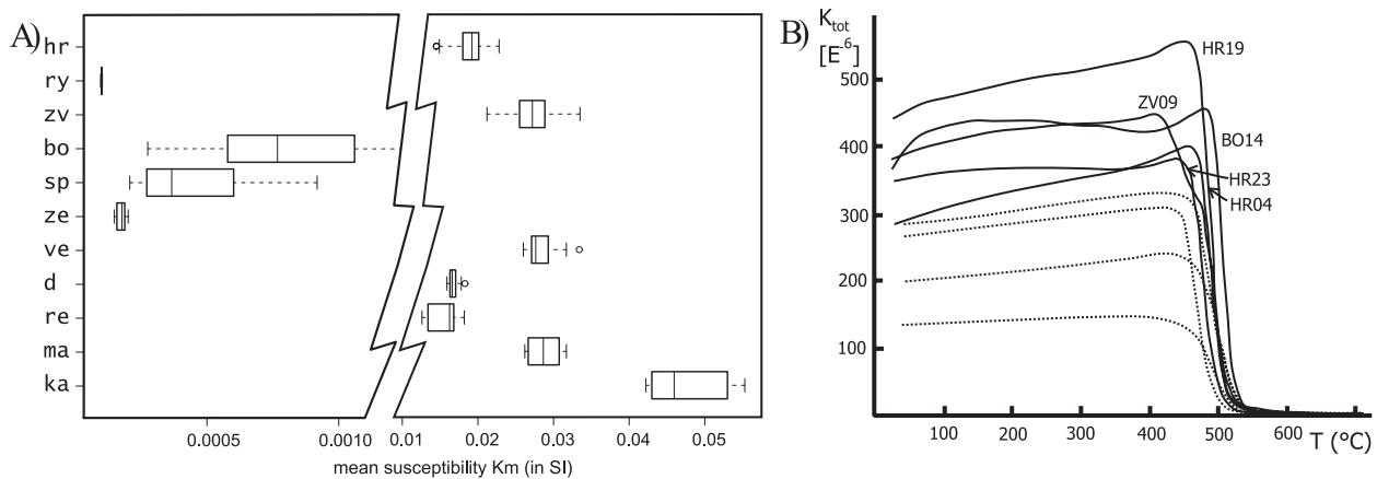
**Fig. 3.** AMS characteristics and magnetic mineralogy. A) Diagram of medians and first and third quartils (boxplot) showing distribution of mean susceptibility ( $K_m$ ) in studied volcanics. B) Thermomagnetic curves of selected volcanoes.
