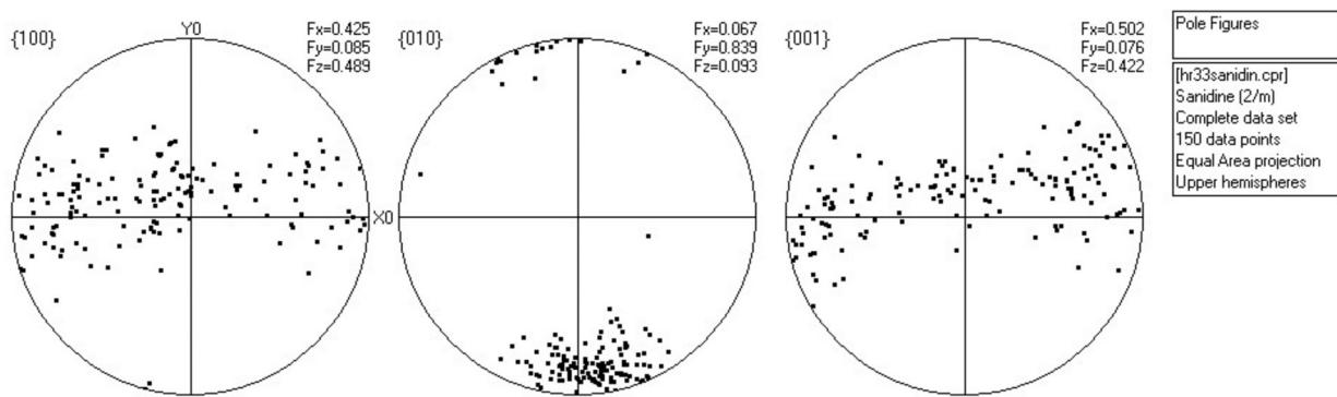
**Fig. 8.** Stereographic projection of  $<100>$ ,  $<010>$  and  $<001>$  directions of 150 sanidine crystals. Sample 33, Hradiště u Habří, Measured by Jakub Haloda.
