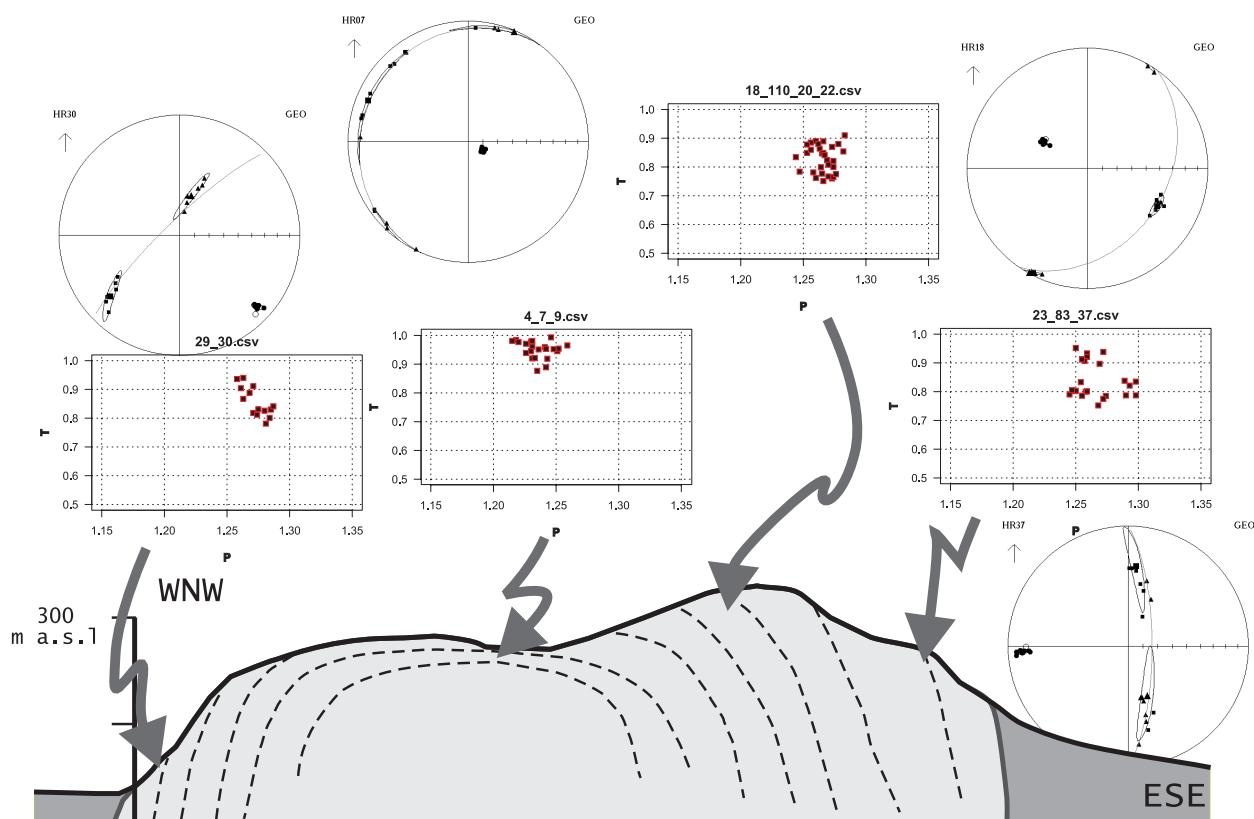
**Fig. 12.** Cross-section of the Hradiště dome showing characteristic AMS fabric patterns including K<sub>1</sub>, K<sub>2</sub>, K<sub>3</sub> axes orientations and P<sub>j</sub>-T plots.
