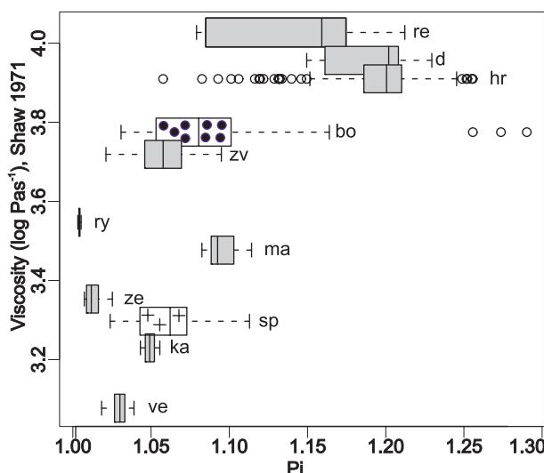
Fig. 6. Diagram of calculated viscosities of magmatic silicate liquids for studied volcanics versus degree of anisotropy expressed in  $P_j$  parameter of Jelínek (1981).
