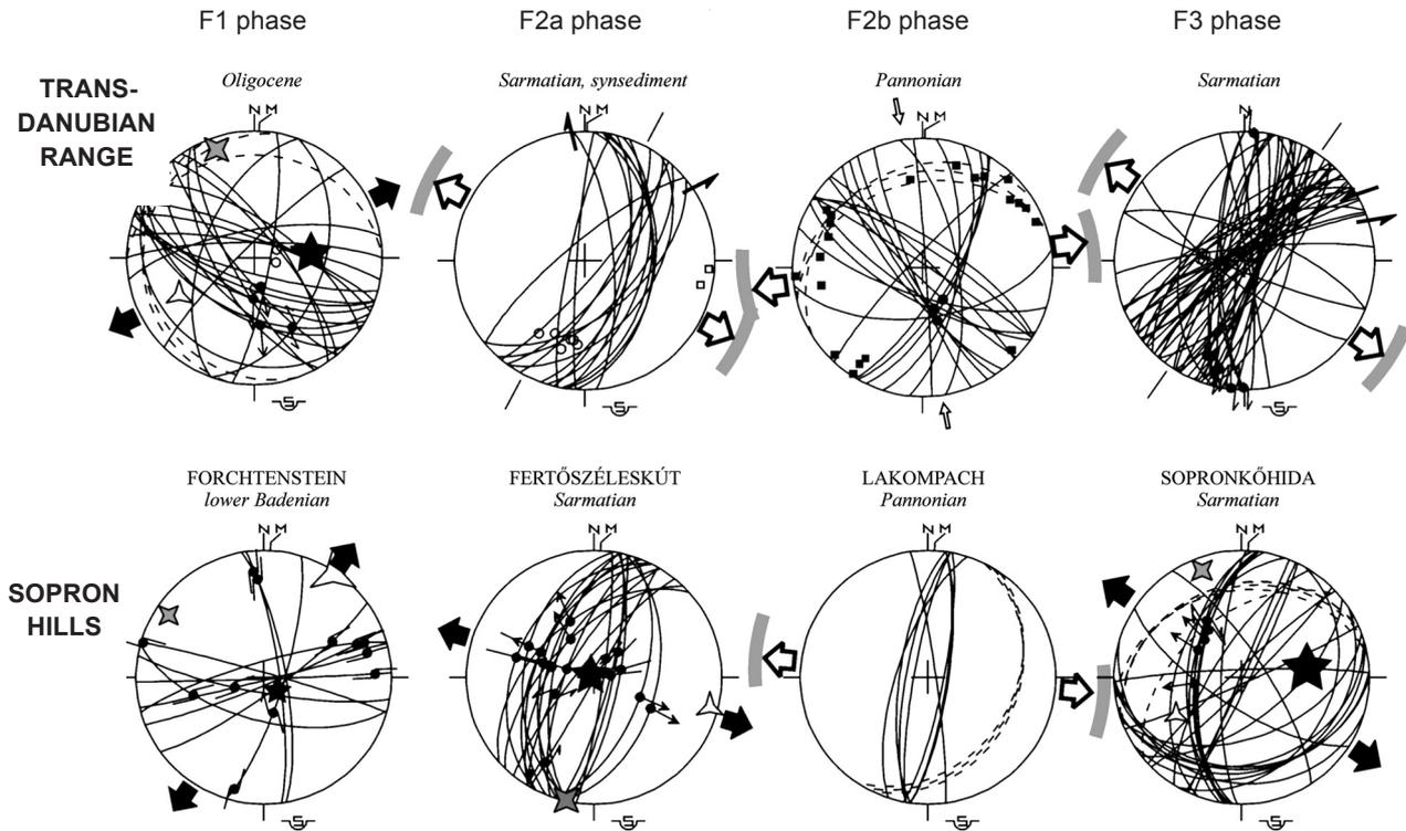
■ **Fig. 1.** The fault pattern and stress field in the Transdanubian Range and Sopron Hills. Stars with three, four and five branches correspond to principal stress axes ( $\sigma_3$ ,  $\sigma_2$ ,  $\sigma_1$ ). The grey arrows correspond to estimated stress axes.
