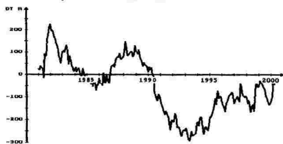
Fig. 9. Integral curve of the monthly precipitation totals (January 1981–April 2000, Bohemia). DT R - precipitation deviation totals.
