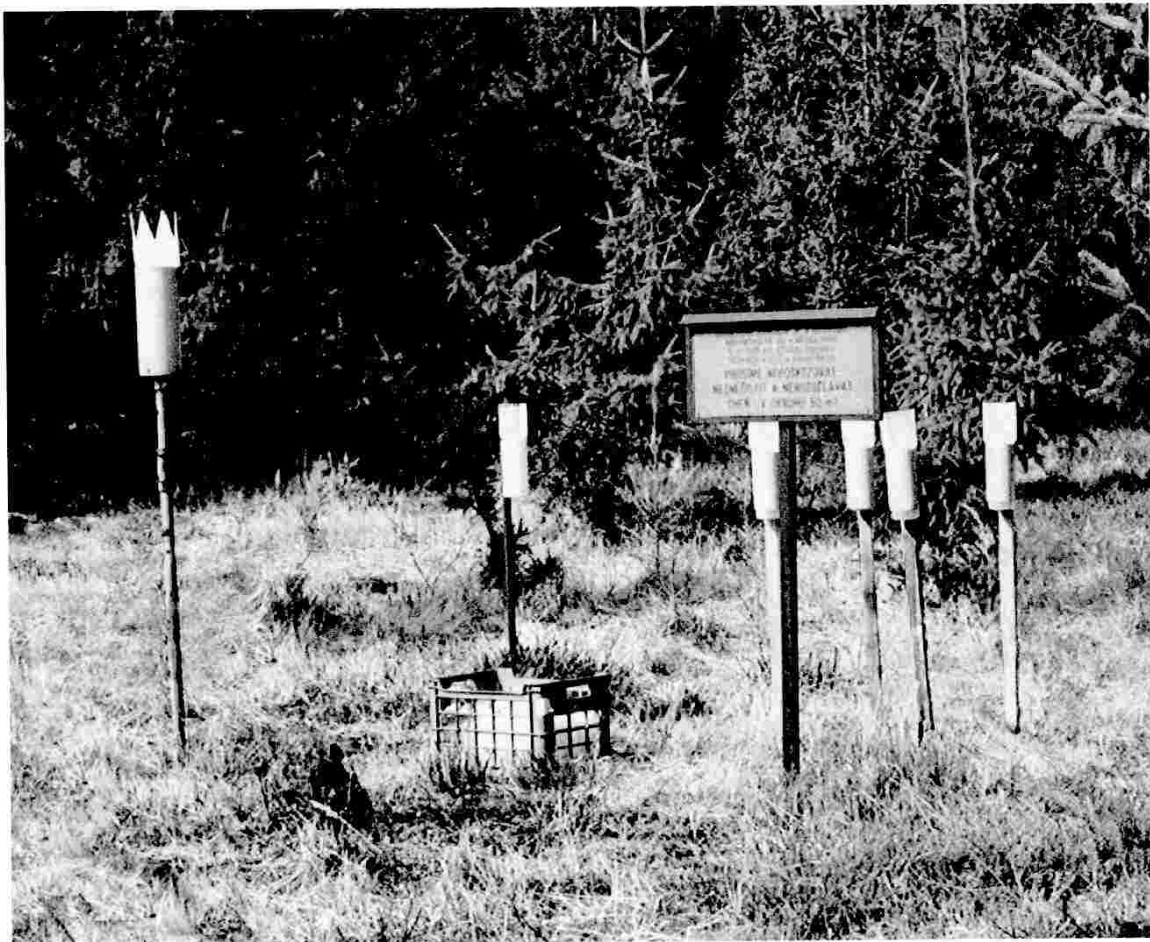
Fig. 4. Collector for the bulk precipitation sampling at Truba.
